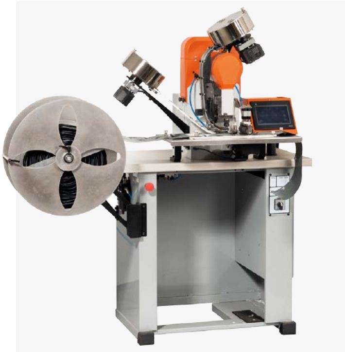
GM250 Eyelet machine with automatic roll up system
