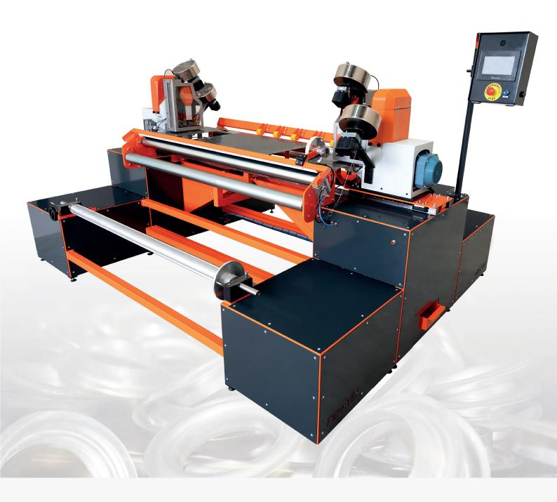
Eyelet Sizes Capacity Metal / Plastic eyelets Eyelets 10 mm - 66 mm Approx. 1800 p/hour Power 380V
