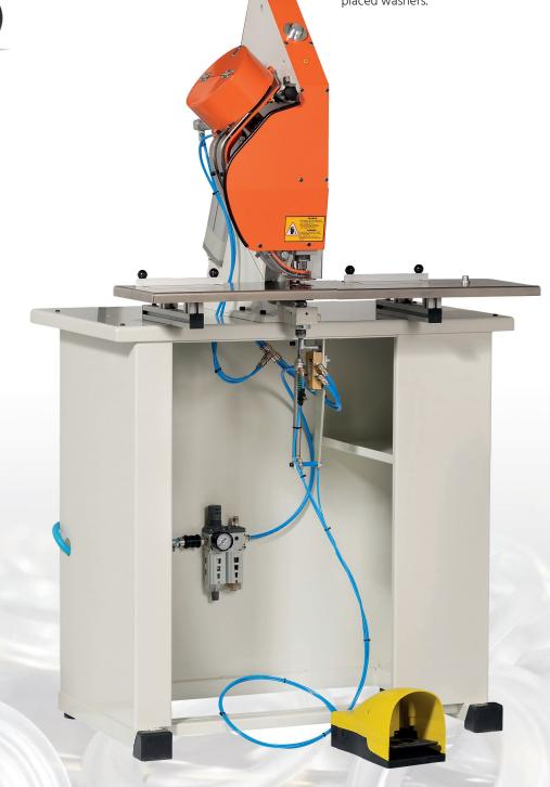
Eyelet Sizes Capacity Oval eyelets 17x11 / 22x14 | DIN 17x11 / 22,5x13,5 Approx. 1200 p/hour
