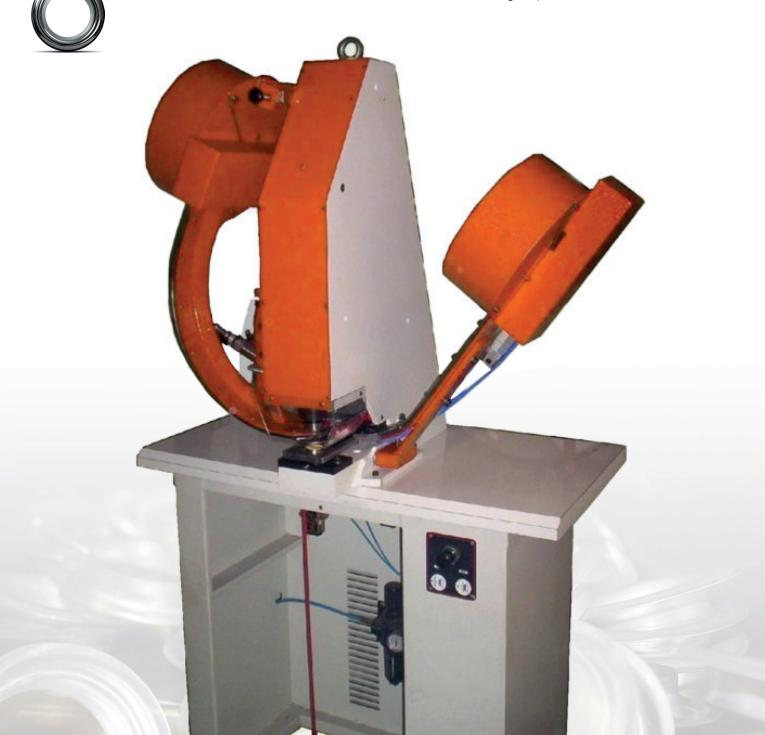
Eyelet Sizes Capacity Metal eyelets Eyelets 25 mm / 40 mm Approx. 800 p/hour Power 230V
