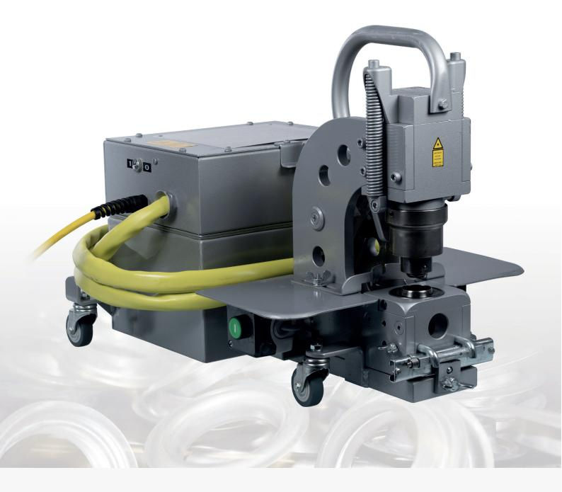
Eyelet Sizes Capacity Metal / Oval eyelets Eyelets 12 mm - 40 mm Approx. 200 - 250 p/hour SupplyHydraulicOperationHandWorking depth7 cm
