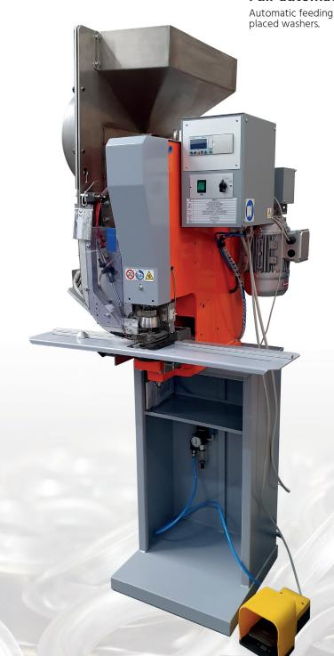
Eyelet Sizes Capacity Metal eyelets Eyelets 40 mm Approx. 800 p/hour
