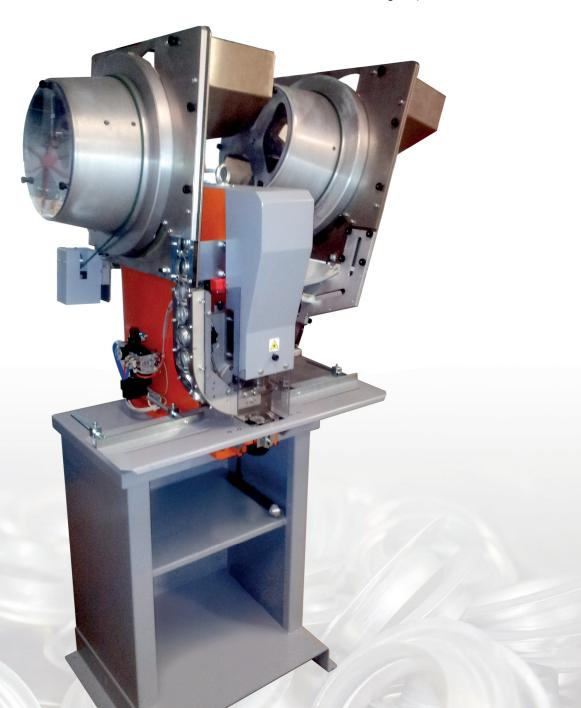
Eyelet Sizes Capacity Metal eyelets Eyelets 25 mm / 40 mm Approx. 800 - 1000 p/hour Power 230V
