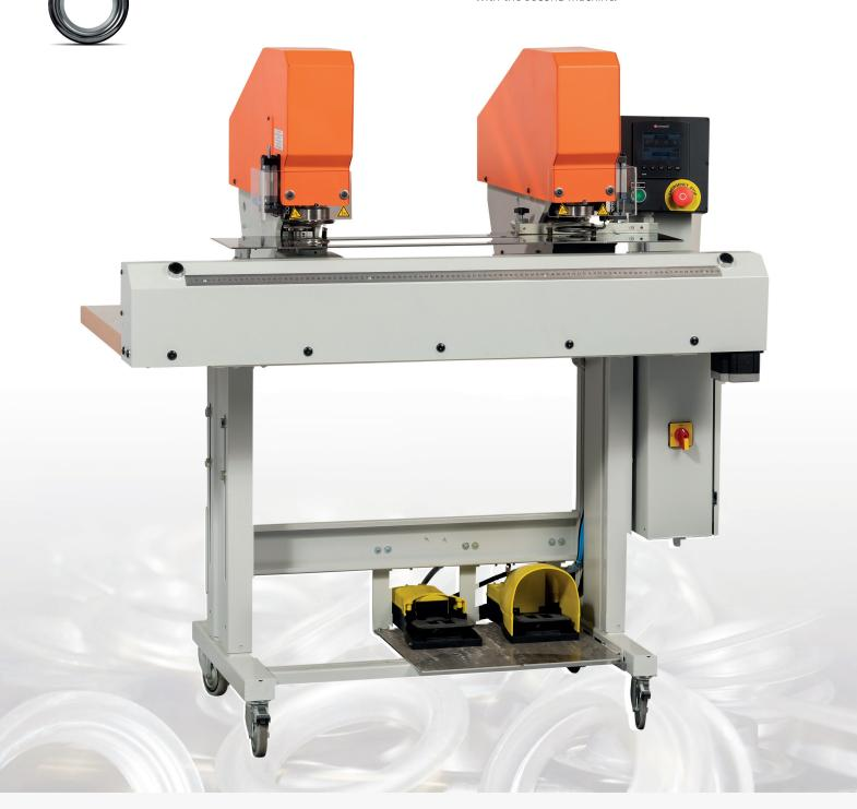
Eyelet Sizes Capacity Plastic eyelets Eyelets 25 & 40 mm Approx. 300 - 350 p/hour Power 230V
