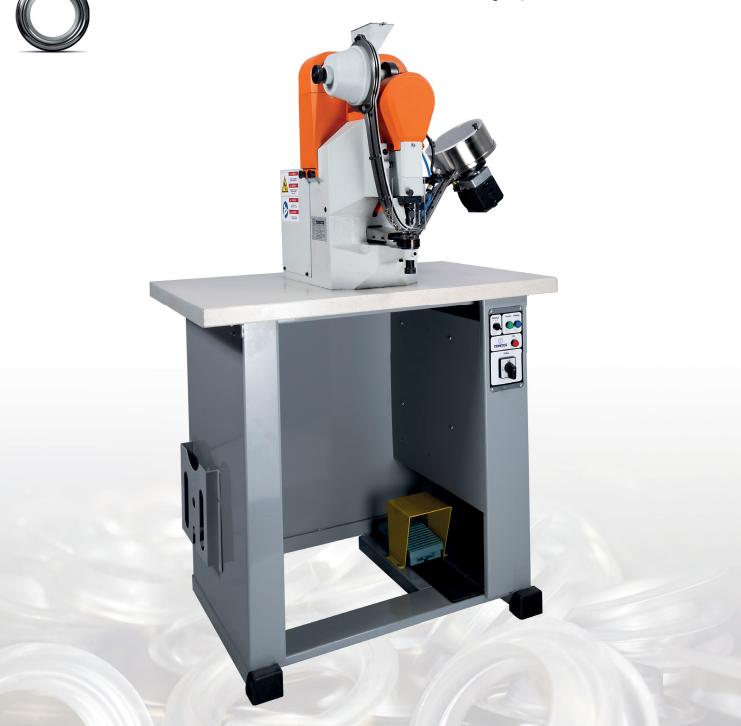
Eyelet Sizes Capacity Metal eyelets Eyelets 4 mm - 8 mm Approx. 1800 p/hour Power 230V
