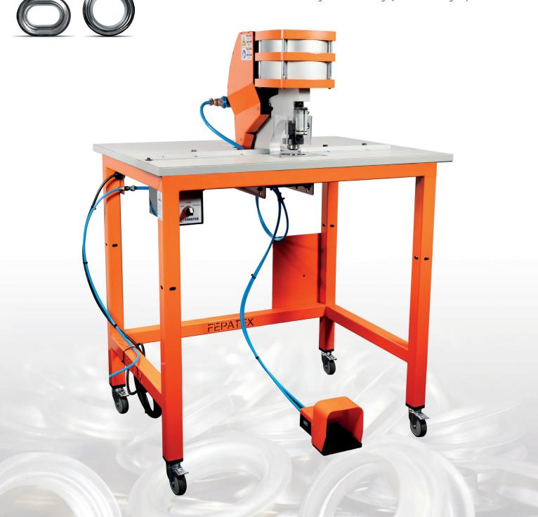
Eyelet Sizes Capacity Metal / Oval / Plastic eyelets Eyelets 10 mm - 66 mm Approx. 200 - 250 p/hour **Supply** Pneumatic (6 BAR) **Operation** Footpedal
