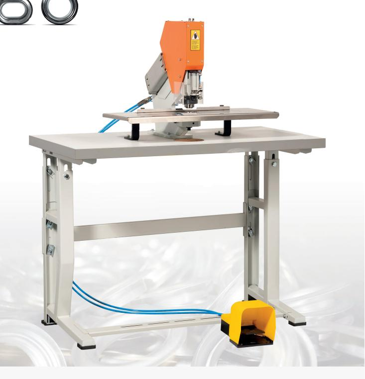
Eyelet Sizes Capacity Metal / Oval eyelets Eyelets 10 mm - 40 mm Approx. 200 - 250 p/hour Supply Operation Working depth
