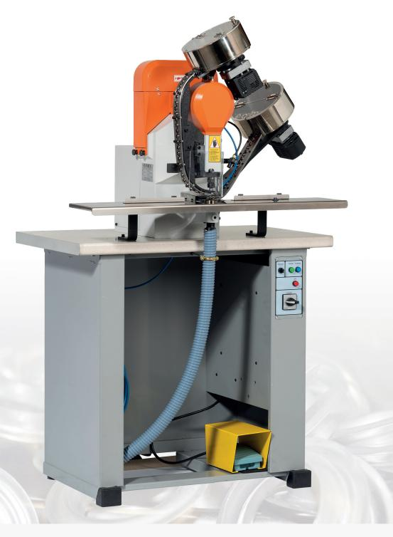
Eyelet Sizes Capacity Metal / Plastic eyelets Eyelets 10 mm - 16 mm Approx. 1800 p/hour
