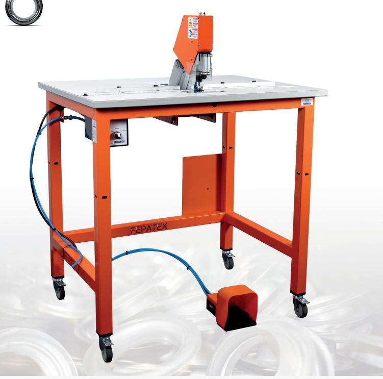
Eyelet Sizes Capacity Metal / Plastic eyelets Eyelets 10 mm - 16 mm Approx. 200 - 250 p/hour Supply Operation Working depth Pneumatic (6 BAR) Footpedal 5 cm
